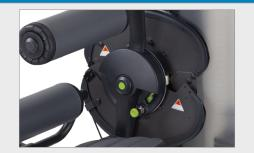
Dual cam system improves biomechanics and reduces cable slack
